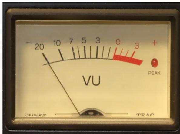
VU Meter: A needle based audio level display
